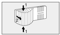
Press the sides of the lamp cover inwards, disengage the cover and unclip it at the rear. ■ Replace the lamp.
